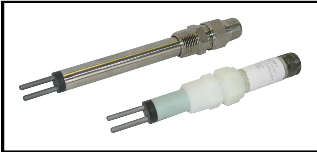
Figure 3 Model 7012 and 6112 Probes
