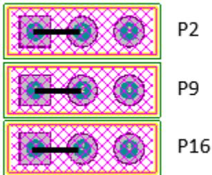
To select the internal, ÅirIQ powered option for each loop, connect jumper pins 2 and 3 as shown below:
