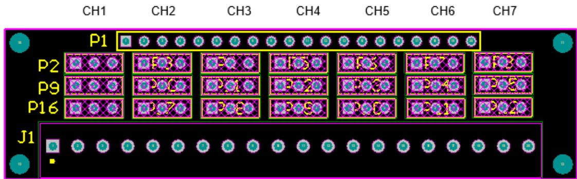
To select the external power option for each loop, connect jumper pins 1 and 2 as shown below:
