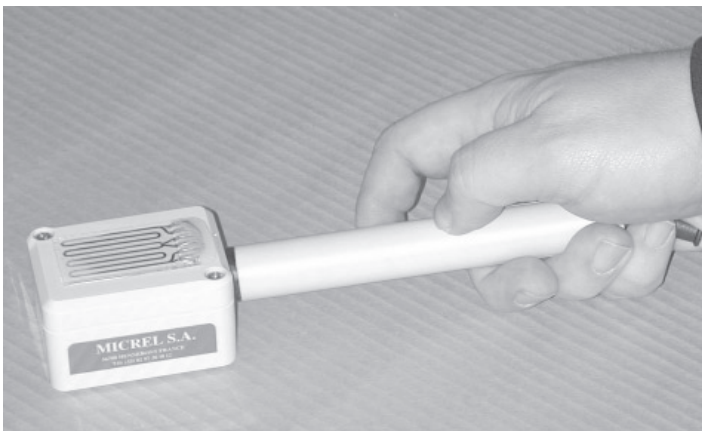
17.3 Taking readings from a prototype corrosion logger.
