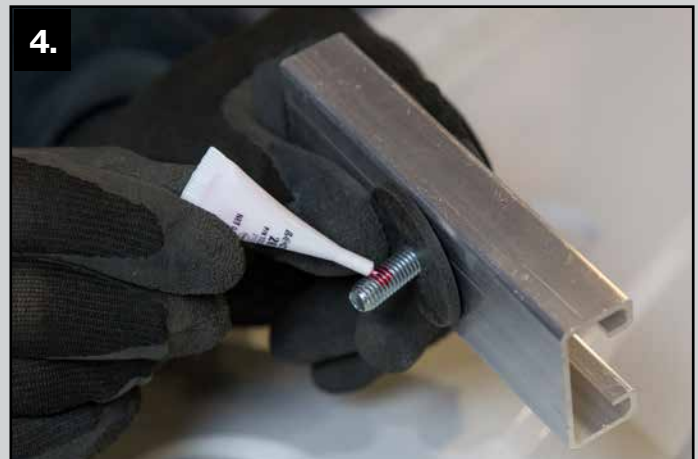
4. Install rubber fender washer over 8 mm bolt. Put a few drops of red Lok-Tite thread locker on the 8 mm bolt threads.
