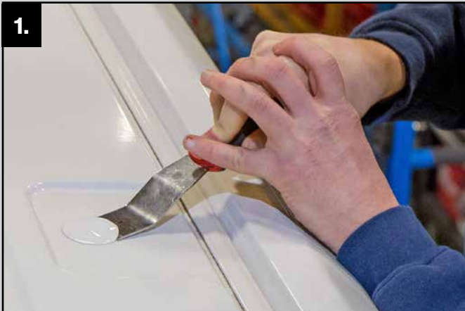
1. Carefully remove rubber plugs for the openings.
