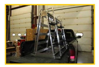
• Drill through the marked mounting locations and secure the rack using the supplied 3/8" hardware
