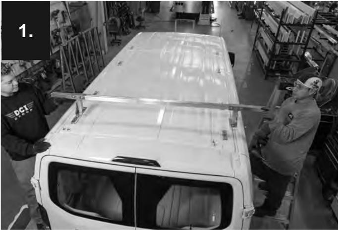
1. Slide 75" crossbars through openings of roof rack mounts so they protrude evenly on either side of the roof mounts.
