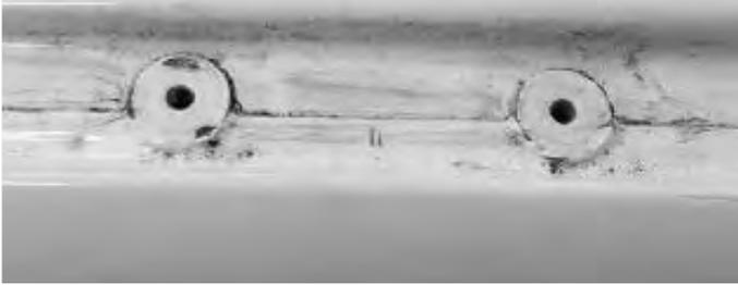
1. Remove plastic plugs from where the roof mounts will be located. (12 plugs total)
