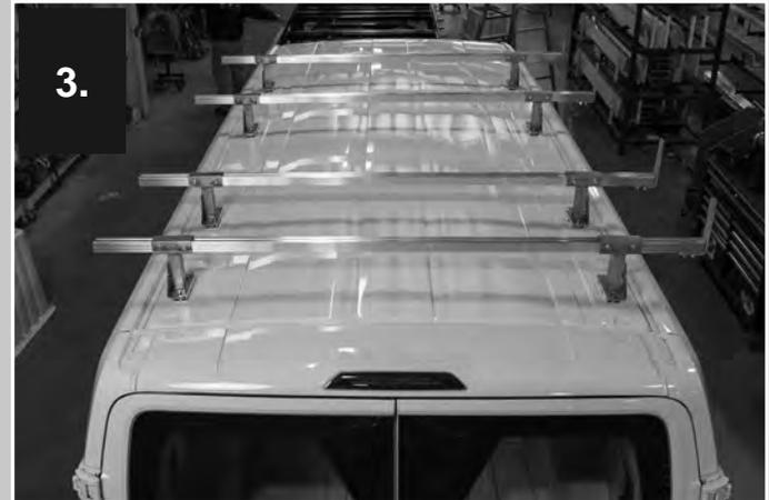
3. Use 5/16" x 2-1/4" bolts, washers and lock-nuts from hardware bag V-8 to fasten crossbars. **NOTE:** Do not tighten bolts fully until crossbars are in final position.
