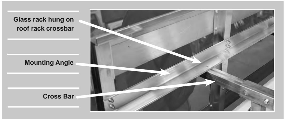
Drill  $3/8$ " holes through the angle and the crossbar, be sure to drill through the center of the angle on the back of the glass rack. Bolt the rack to the each of the cross bars using the  $3/8$ " x  $2-1/2$ " bolts from hardware bag V-10.
