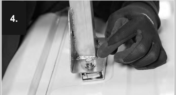
4. Loosely secure roof rack mounts to adapter using M6 bolts with washers and lock washers from the hardware bag for roof rack mounts. It's important that the tall roof mounts are located at the rear of the van.
