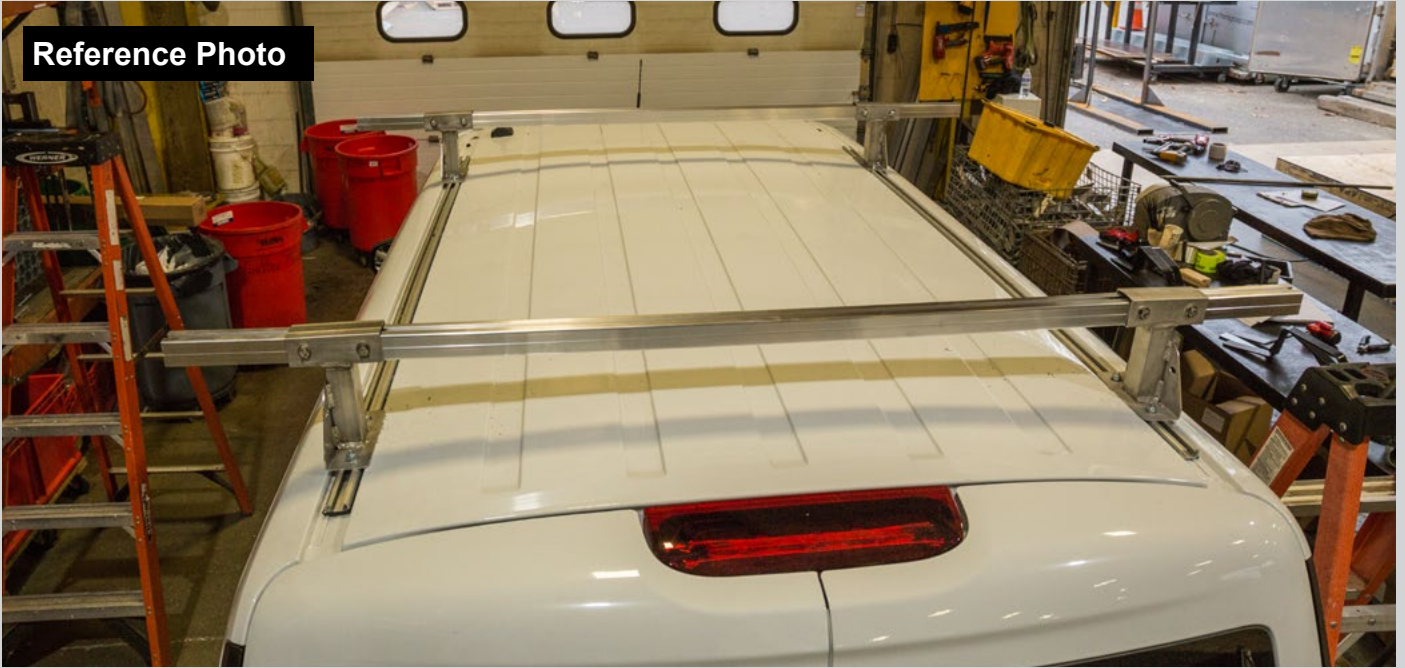
Completed Roof Rack Installation
