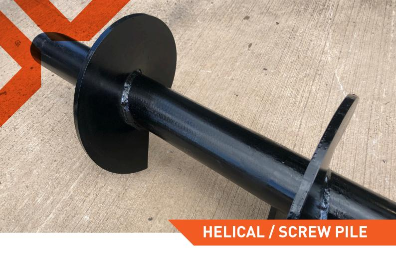
Helical Piles or Screw Piles are steel tubulars that have had helix/helix's welded to them to allow the pile to be screwed into the ground. We use our high-quality repurposed steel tubulars for these piles and so the piles can benefit from the carbon saving that this offers. The piles are made in-house and manufactured to the requirements of the client.
