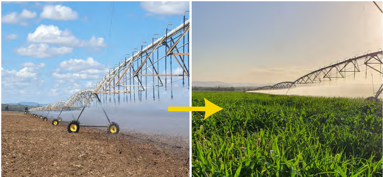
The above image shows a recently installed pivot at Comanche (left) and forage sorghum growing under the pivot (right). Centre pivots are irrigation systems which irrigate crops in a circular pattern and are capable of applying water and fertiliser. This type of irrigation system is efficient and effective as it can apply a precise amount of water calibrated to the needs of the crop. Most systems have the capability of delivering up to 16mm per day.
