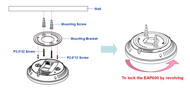
3) Mount the EAP600 on the mounting bracket by rotating the unit clockwise about 90 degrees to secure it in place.
