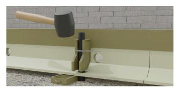
Push clamp bodies down hard, so that teeth on the bottom engage and interlock in the ridges on the rail base, then tighten zip tie to prevent clamp body moving.
