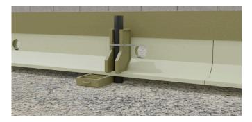
8. Tap clamp body gently down to ensure a secure fixing, if using the larger rails, a pair of wedges can be inserted between the vertical blade and the clamp body or pin, to stiffen and avoid bending of the blade if required, for when large vibrating screed machines run along it.
