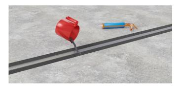
11. With the slabs/screeds now installed and hardened, if a joint filler is to be used, simply remove the caps and "hook" out the ferrules, then pour the flexible joint filler into the top void of the rails, level with the slabs/screeds.
