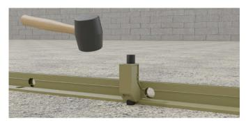
6. Position pins in holes or larger rails, or close to the rail base edge on the small rail, drive into sub base to desired depth.
