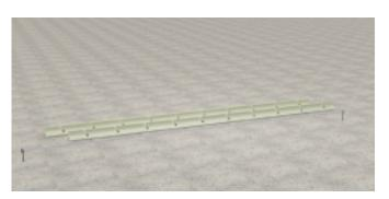
1. Place string-line along where the Tec-Form is to be positioned.
