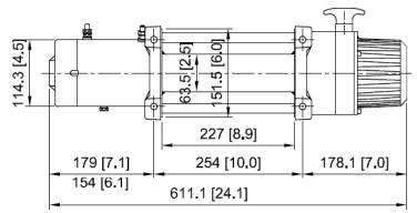
NB: Neither the roller fairlead nor the solenoid enclosure mount to the winch.
