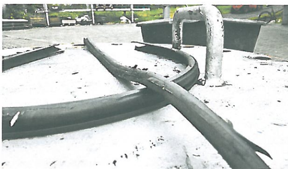
Gasket removed out from Cover lid and Clamp (before Test No.5)
