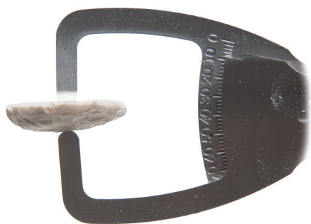
Fig. 29: Use the Patella Calipers to determine maximum thickness
