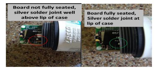
When replacing the cap, first check that the sensor board is inserted all the way into the unit, and that no wires will be pinched. With OLDER mounting styles, the silver bead on the antenna will be your guide. With new, taller caps, the backboard rests on the TOP of the threads, ensuring clearance.
