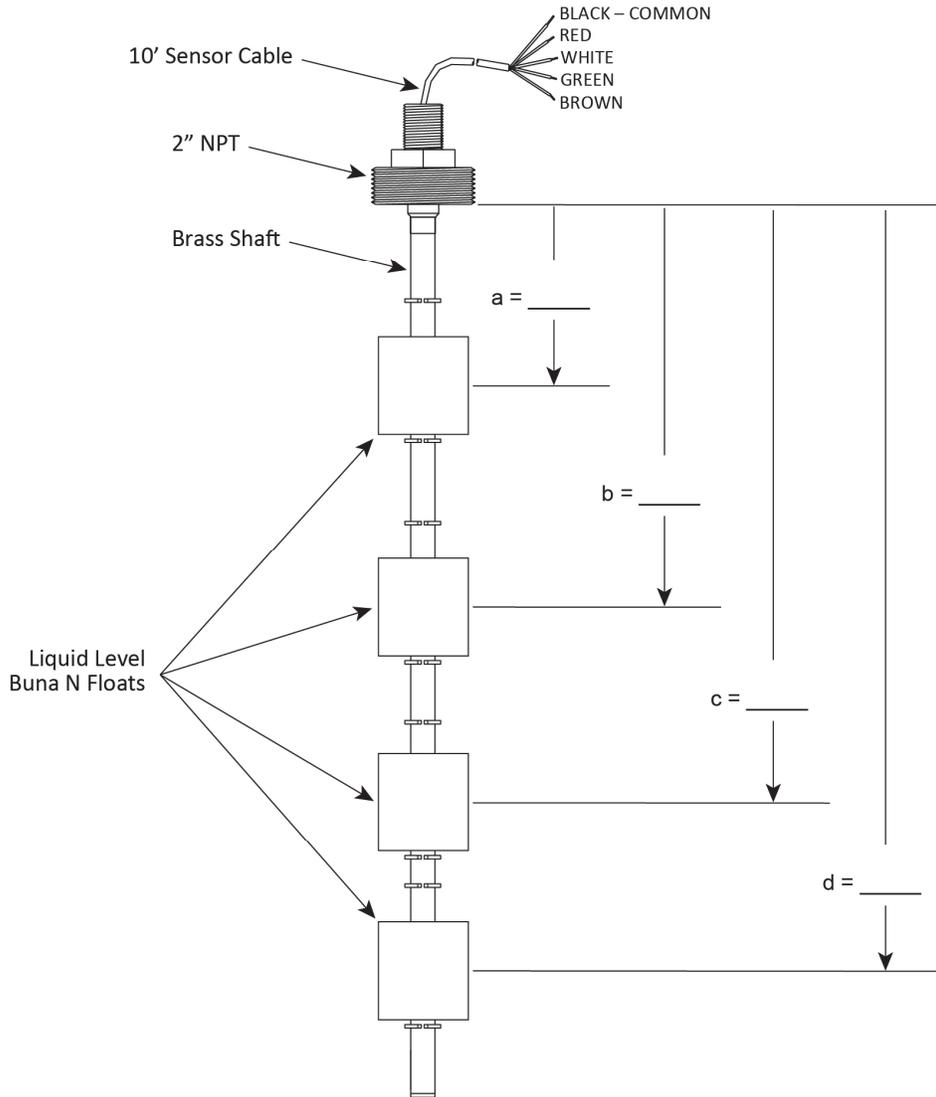
**IMPORTANT:** Dimensions should be calculated from the top of the tank or riser down to the required alarm level(s) in inches. Be sure to take into account any riser pipes or manway risers.
