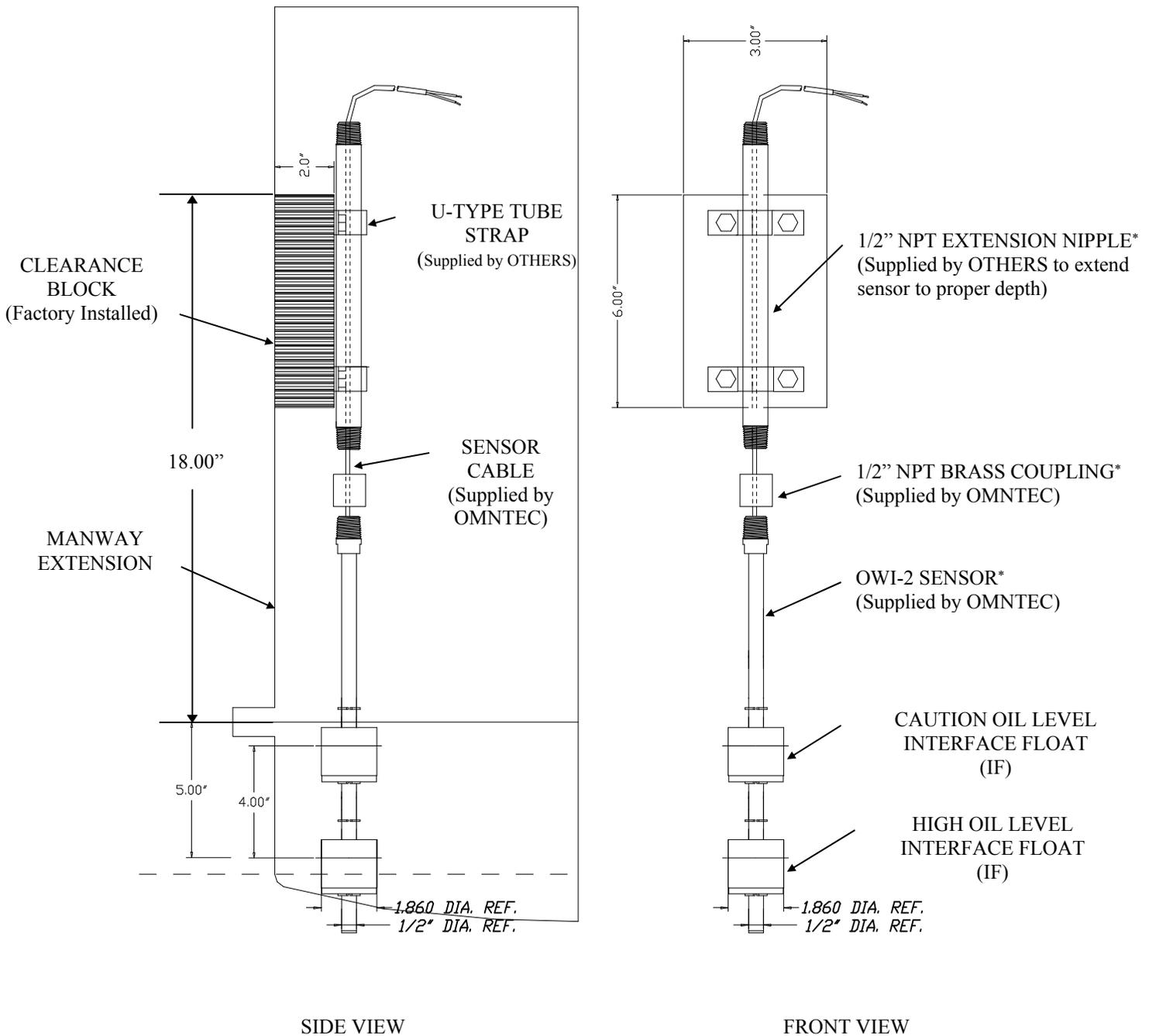
**\* WARNING-** It is the installer's responsibility to select a thread sealant that is compatible with the product being stored and that all NPT fittings are fastened properly to assure liquid tight seal for proper sensor operation.
