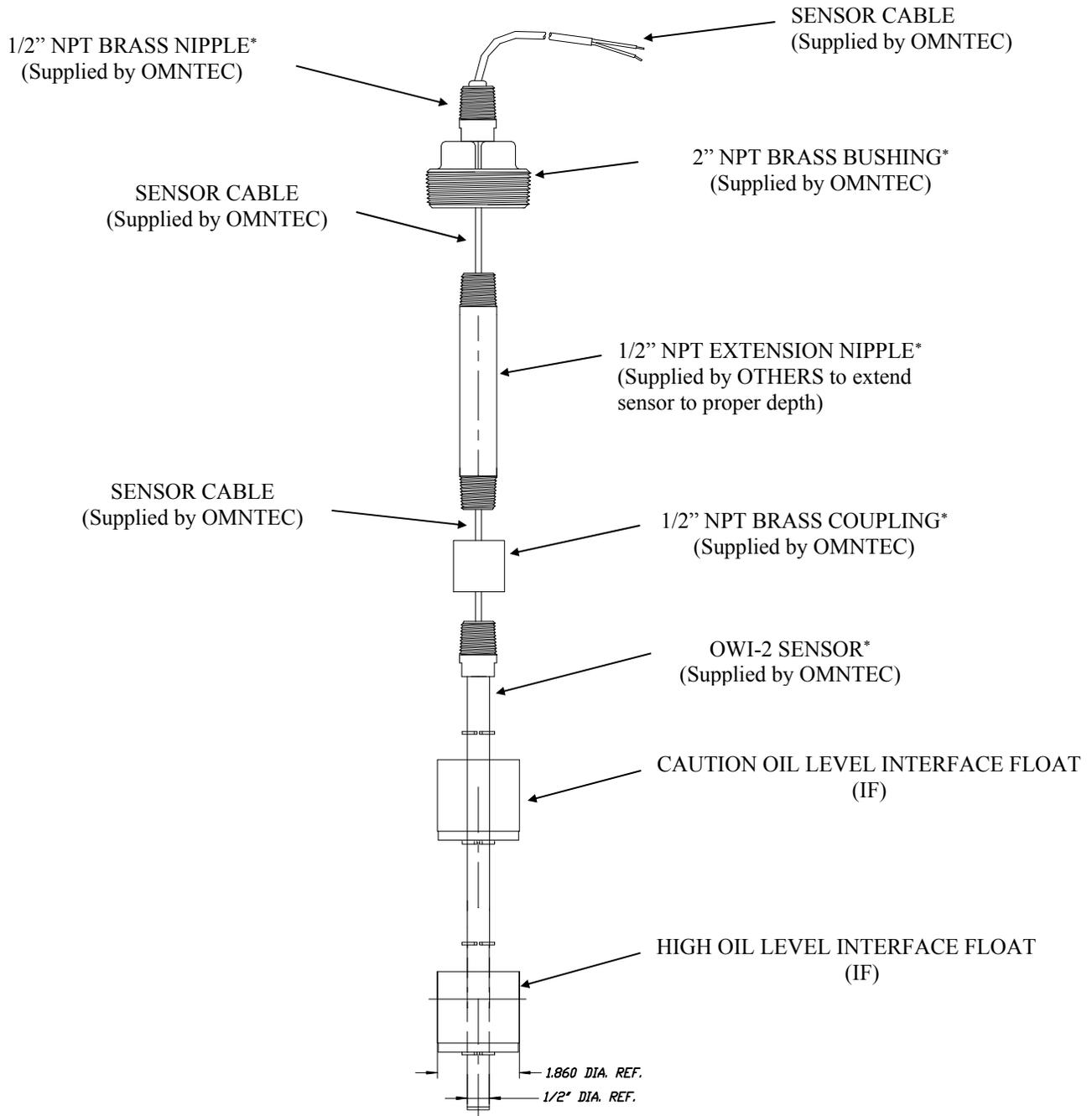
\* **WARNING-** It is the installer's responsibility to select a thread sealant that is compatible with the product being stored and that all NPT fittings are fastened properly to assure liquid tight seal for proper sensor operation.
