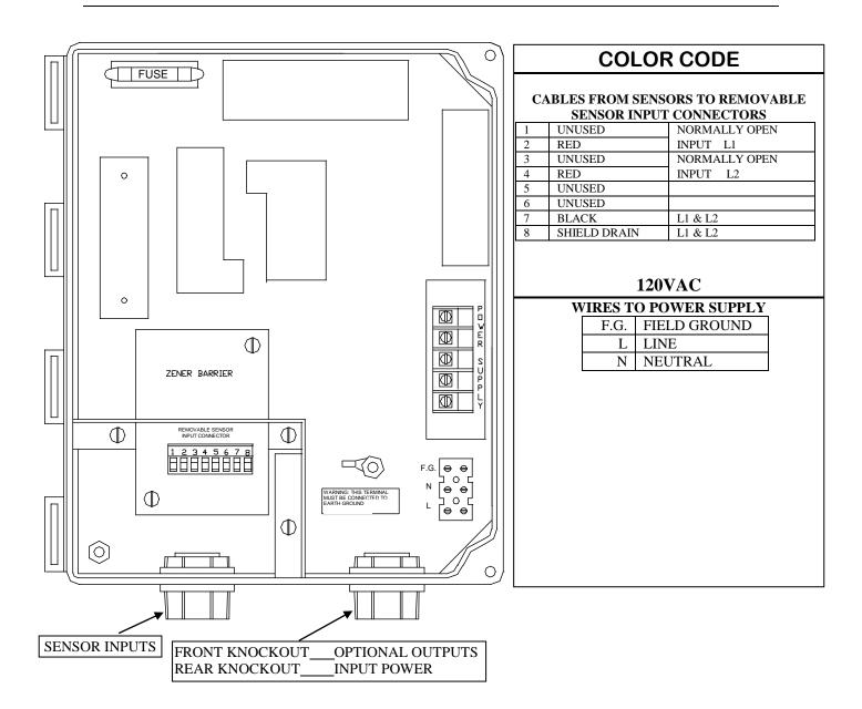
NOTE: To maintain proper shielding, <u>BLACK sensor wires</u> and SHIELD DRAINS should **not** be connected together at sensors.
