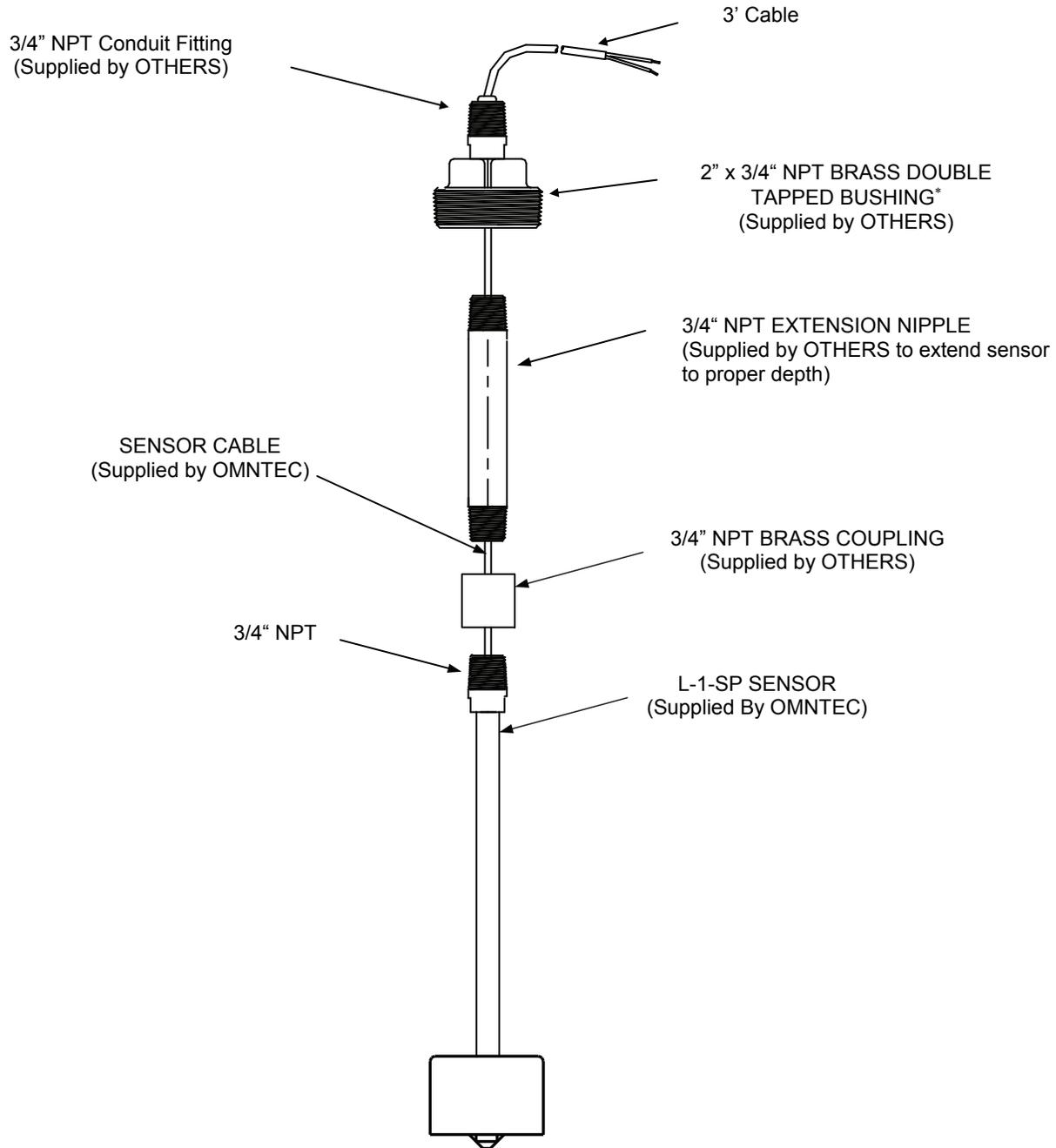
**\*WARNING-** It is the installer's responsibility to select a thread sealant that is compatible with the product being stored and that all NPT fittings are fastened properly to assure liquid tight seal for proper sensor operation.
