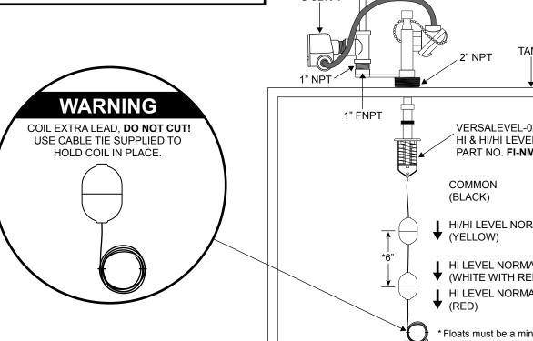
PART NO. DC-TX-D1 U-JBK-1 **TANK** VERSALEVEL-02 HI & HI/HI LEVEL SENSOR PART NO. FI-NM-V2-M-160" HI/HI LEVEL NORMALLY CLOSED HI LEVEL NORMALLY OPEN (WHITE WITH RED STRIPE) HI LEVEL NORMALLY CLOSED \* Floats must be a minimum of 6" apart from each other. MAKE SURE TOP OF TANK IS FREE OF ANY OBSTRUCTIONS TO PROMOTE FREE MOVEMENT OF COIL.
