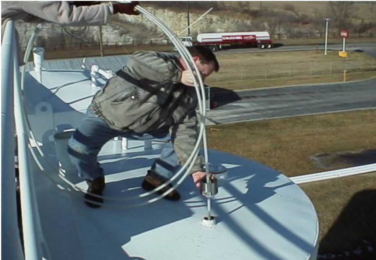
Figure 20 – Feeding DataStik™ Probe Into Tank (VB Model shown)
