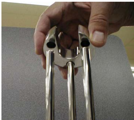
Figure 41 – Installing Spring into Half Cap Brackets
