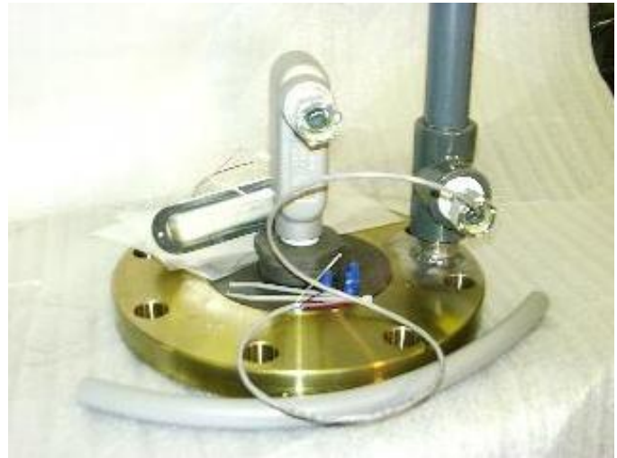
Figure 28 – Fishing Wire Through J-Box
