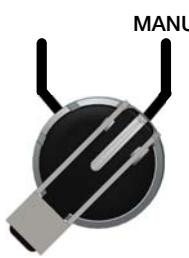
The **MANU** operating mode is available only when the button is unlocked. It gives access to a temporary control of the actuator in 3 modulating points
