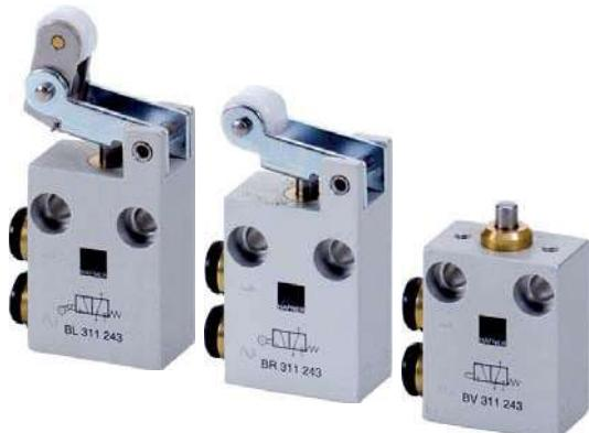
Mechanically actuated 3/2-way spool valve with mechanical spring. Ports 1 and 2 are on one side of the valve, equipped with 4 mm push-in fittings.
