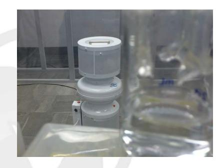
Photographs are the device received by the laboratory on 10 MAR 2016. The device is photographed operating within the chamber and the SKC bio-sampler in the foreground.
