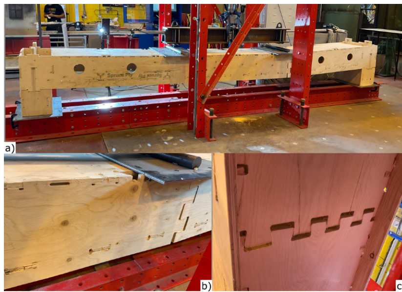
Figure 4: a) Overview, b) detail of stitch joints and side dovetail joints, c) detail of bottom flange dovetail joint.
