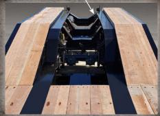
Remove the center bogie section to create a low boom well that is great for hauling excavators—4-point lift system makes it easy to convert.
