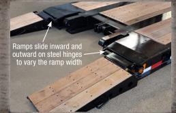
Front flip ramps feature 9° load angle with adjustable widths to handle a wide range of equipment (ramps slide horizontally).
