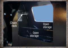
Gooseneck features a generous open storage area accessible from the front or back of gooseneck with chain bar storage and dividers.
