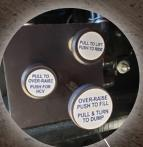
Controls are located for easy access from the rear whether the bogie center section is installed or removed.
