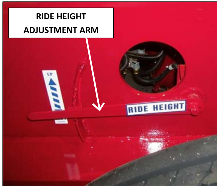
Figure 2-6. Ride Height Adjustment Arm
