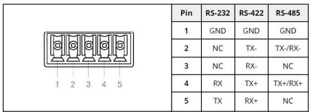
COM terminal pinout
