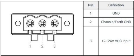
3-Pin terminal power pinout
