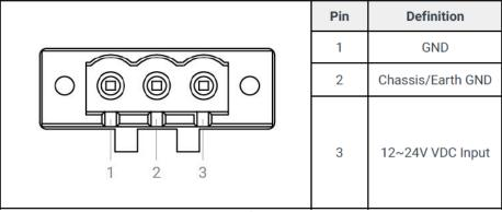
3-Pin terminal power pinout
