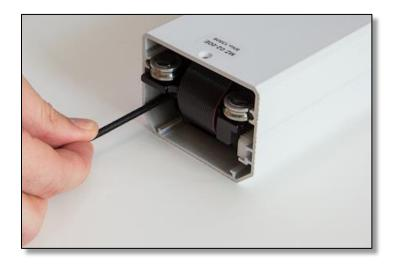
**Step 15:** Connect the long tension cord to the top cover of the injection head. Tighten the screws to secure the cover to the top of the injection head. Required tool: Torx T10
