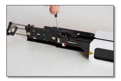
Step 13: Insert the bumper (PAL MZAgiOpen) and tighten the two screws holding it in place.
