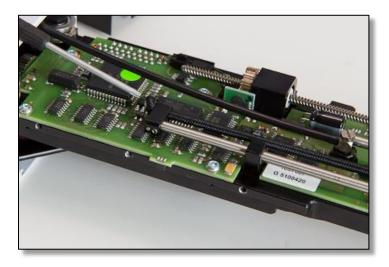
Push up the lower needle guide to the stop to check that the knot of the Tension Cord does not touch the electronic board and that nothing hinders the up and down movement of the needle guide assembly.
