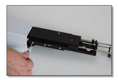
Step 7: Remove the cover to gain access to the electronic and needle guide mechanical part.
