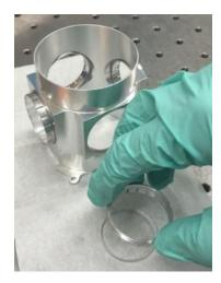
Pressing tension ring onto the window
