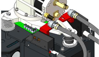
Bracket locked in upward position (for operation)
