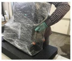
Step 2: Sliding out the cryostat
