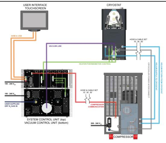
1. Remove any plastic covers from the connector locations on the back of the compressor, the cryostat, the system control unit, and the vacuum control unit.
