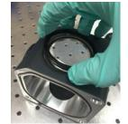
Step 3: Removing retaining ring
