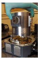
Step 4: Lifting off radiation shield assembly
