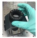
Step 1-2: Using window tool to unscrew retaining ring
