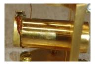
Step 3a: Thermometer clamped to mounting surface
