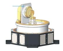
Step 3b: fixed side of radiation shield stays in place (indicated with blue arrow)
