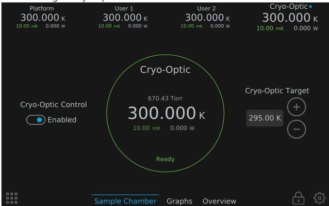
Before cooling down the system, the Cryo-Optic temperature channel must be enabled.
