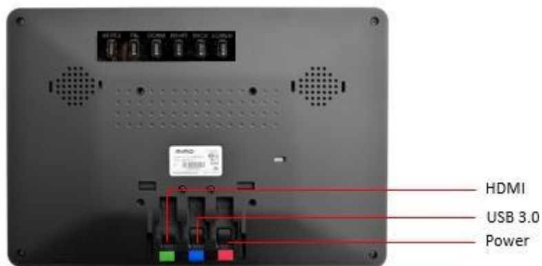
Figure 7: Touchscreen monitor inputs.
