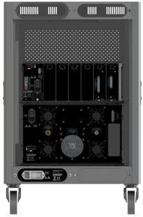
Cart with Electronics Rack (rear view shown with VC1110 bottom and SC1160 top)
