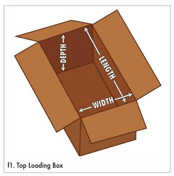
If measuring the inside of an existing box, make sure to measure from the center of the score (the crushed fold line). A good trick is to fold the board inward and draw a line in the crease. Then measure from the drawn line, to line.
