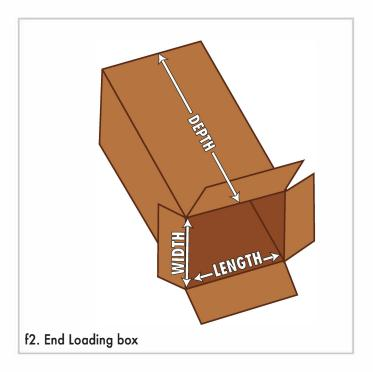
We refer to the inside dimensions because the corrugated board thickness may vary. A box constructed of B flute will not have the same outer dimension as a box made from E flute.
