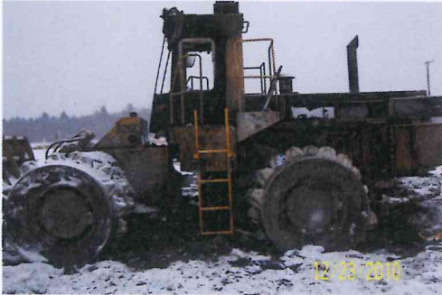
Fig. 1 Burned out compactor Dec. 2010
