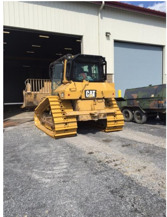
Fig. 4 – D6 dozer with new tracks rollers, chains and sprockets ready to return to work
