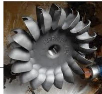
A photograph of a large, metallic Pelton turbine runner with a distinct fan-like shape, resting on a surface. |
