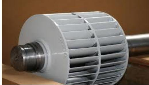
A close-up photograph of a white, multi-bladed cross-flow turbine runner mounted on a shaft.                   |
