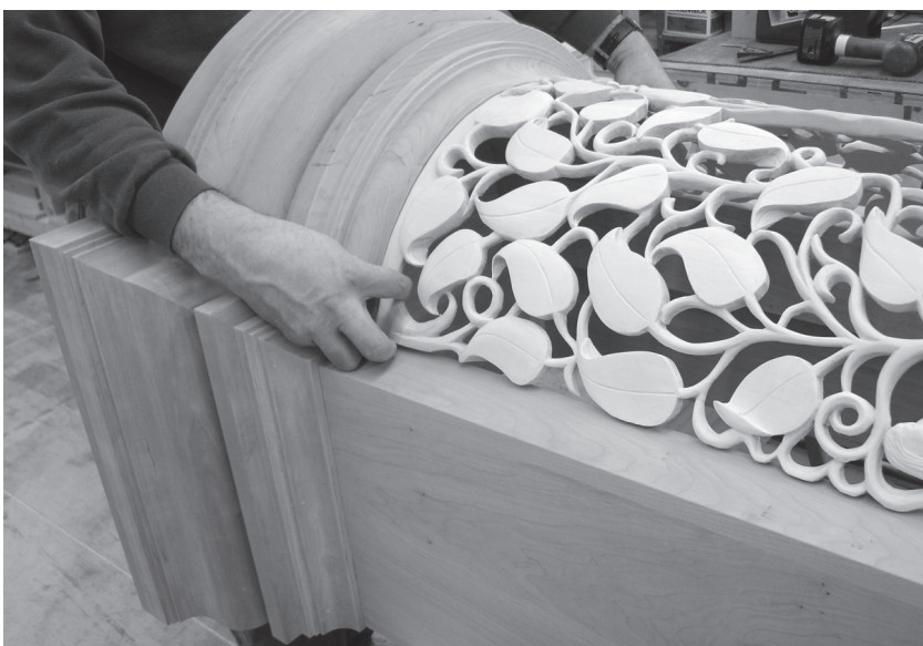
Pipe shade being fitted in the Kegg shop
