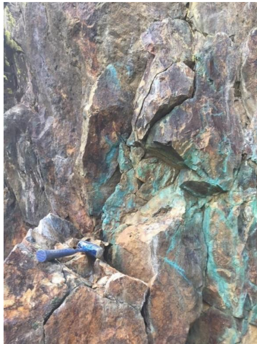
Figure 9-8 Significant CuOx and Erythrite Coating on the outcrop surface near Upper Ludwig Adit
