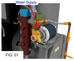
On models furnished with condensate return tank, connect water line to makeup valve located at tank end. (See Instruction Supplement 1 in this manual) R, RH and RHC steam boiler models require four (4) gallons of feed water per hour for each 10 kW of electric heating capacity of the boiler. Lines should be of adequate size and meet local plumbing codes.
