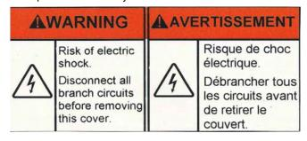
Located on end caps of cylindrical boiler pressure vessel jacket
