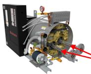
Use a stiff wire brush to remove all scale and foreign matter from the element rods.
