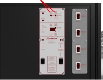
As soon as no boiler alarms are indicated, the HEATING light turns on and the boiler starts to build up pressure. Observe the pressure gauge while pressure builds up, until working pressure is reached. The working pressure should have been factory set to your specification. However, if you wish to change the working pressure setting, proceed as follows.
