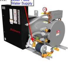
On models furnished with condensate return tank, connect water line to makeup valve located at tank end. (See Instruction Supplement 1 in this manual) R, RH and RHC steam boiler models require four (4) gallons of feed water per hour for each 10 kW of electric heating capacity of the boiler. Lines should be of adequate size and meet local plumbing codes.
