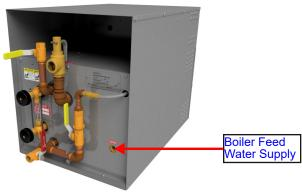
On models furnished with condensate return tank, connect water line to makeup valve located at tank end. (See Instruction Supplement 1 in this manual) R, RH and RHC steam boiler models require four (4) gallons of feed water per hour for each 10 kW of electric heating capacity of the boiler. Lines should be of adequate size and meet local plumbing codes.
