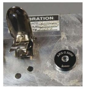
This 2.5-mm-diameter cubic zirconia ring gage was purchased for a job that required bores with particularly tight tolerances. Calibrating the CMM with artifacts that closely match the size and geometry of measured features is one of many lessons from such work that have translated to the broader shop.
