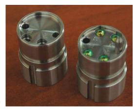
A closer look at the fiber-optic connector inserts. The optical fibers are contained within ceramic sleeves, or ferrules, that fit snugly within 2.5-mm-diameter bores, which feature 3-mm counterbores on the connecting ends to accommodate the lenses.
