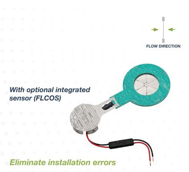
OsecoElfab's FLCO rupture disc is easy to install and non-torque sensitive. The disc fits between standard 150# ANSI RF flanges with no need for a holder. As a flat, bi-directional device with the same burst pressure in either direction, the FLCO cannot be installed incorrectly, eliminating installation errors.
