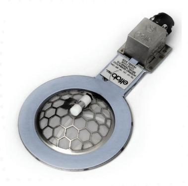
This range of composite, low pressure reverse acting rupture discs are manufactured with integral burst detection. They feature a 5-pin DIN connection and are suitable for applications operating at low pressures.
