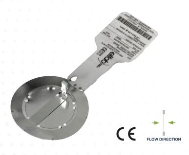
OsecoElfab's Two-Way Flat Composite disc acts as a single design for both positive and negative pressure protection. Manufactured with various slotting arrangements to meet specific application requirements, it is compatible with liquid, gas and vapour applications.
