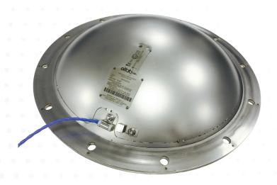
Applications that are maintained at higher temperatures need to retain heat energy while still ensuring safety. Our thermal explosion vent combines a solid thermal insulator of low-density silica within a stainless steel panel construction. The integral insulations prevents loss of heat efficiency while maintaining safe, reliable explosion protection.
