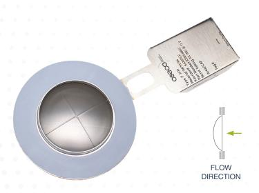
OsecoElfab's ICD from Broken Arrow is scored and used to protect intermodal containers. The ICD utilizes a nickel disc with a 316 Stainless Steel centering ring. The disc also features fluoropolymer gaskets and a fluoropolymer liner on the process side for use in highly corrosive applications.
